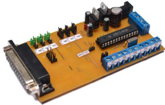
**Fig. 7.** Prototype of evaluation board EVAL USTI-MOB.
