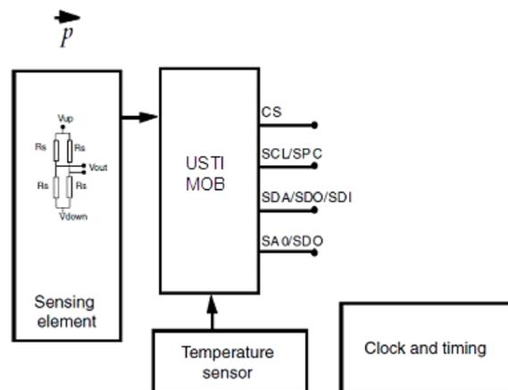
Fig. 4. Barometric pressure sensor based on USTI-MOB IC.
