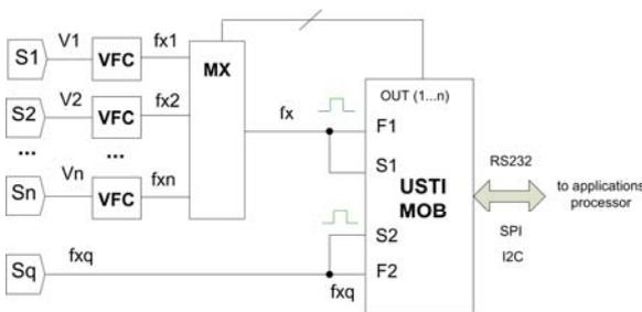
**Fig. 6.** Multisensor system for mobile devices and IoT with analog sensors.
