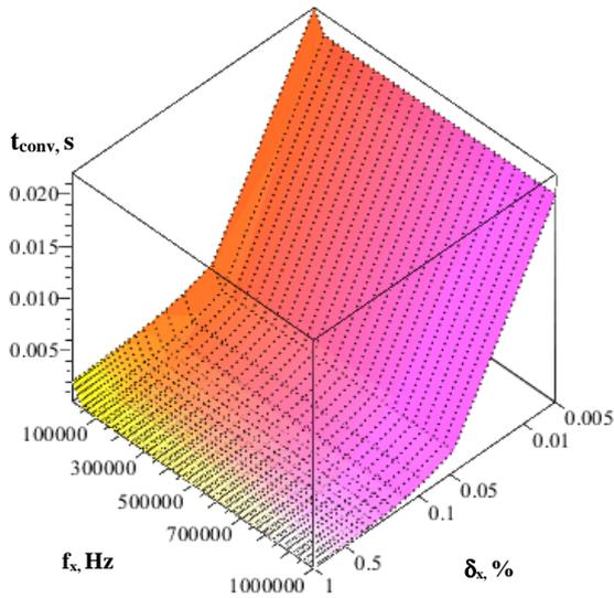
Fig. 8. Dependence of  $t_{conv}$  ( $\delta_x, f_x$ ) in the frequency range from 500 Hz to 1 MHz.
