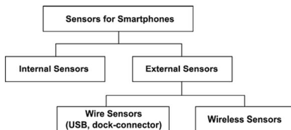
Fig. 1. Smartphone and tablets sensors classification.
