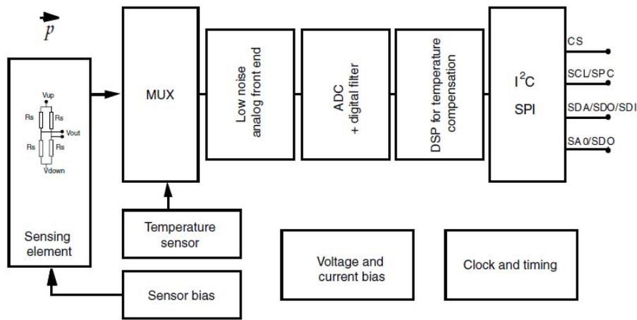
Fig. 3. Barometric pressure sensor based on ADC.
