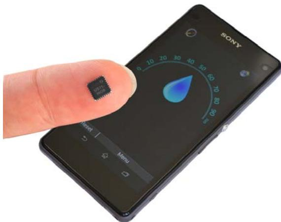
Fig. 9. USTI-MOB IC in  $5 \times 5$  mm MLF package.
