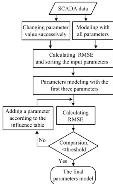
Fig. 4. Flowchart of parameters modeling.
