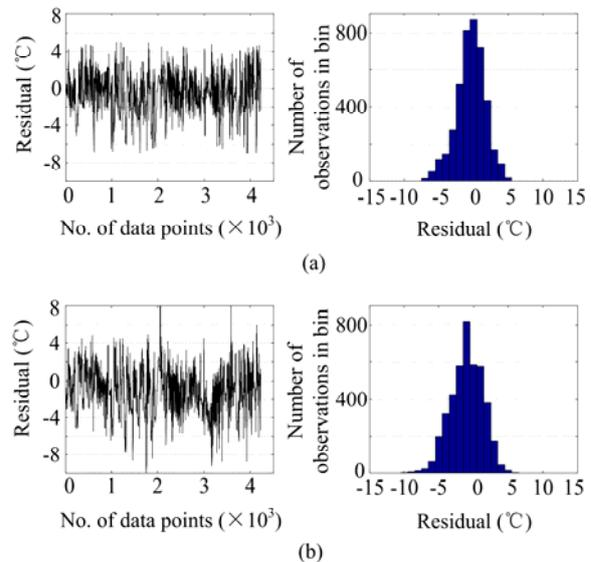
Fig. 5. (a) Residual and distribution of parameter model for temperature of generator bearing B using the proposed method in this paper and (b) the method in [20].
