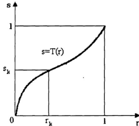
Fig. 2. Histogram equalization transform function.
