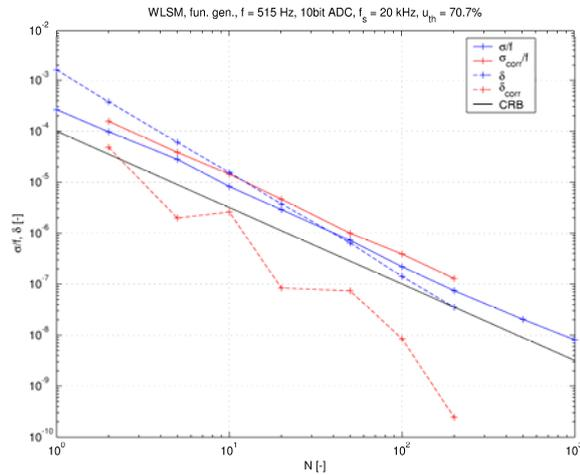
**Fig. 10.** Experimental verification and comparison of the WLSM and double estimation method.
