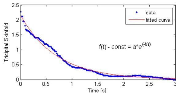
Fig. 8. Example of an excitation step response of a first order system.
