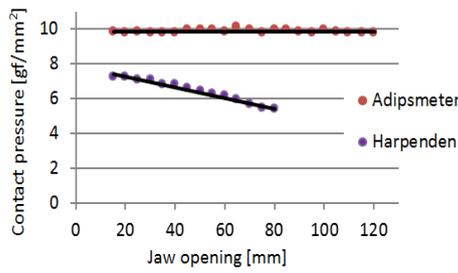
Fig. 5. Pressure test between end tips for different jaw opening.
