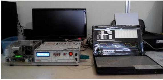
**Fig. 1.** The e-nose apparatus used to analyse sensory response of three varieties of gingers in this study.
