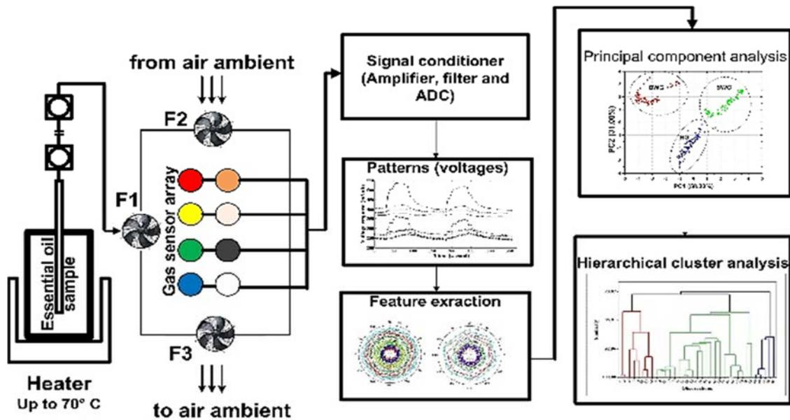
**Fig. 2.** Schematic block diagram of e-nose used in this study.
