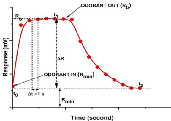
**Fig. 3.** The typical sensor response of a TGS gas sensor while measuring a ginger sample (one cycle consisted of sensing and flushing).
