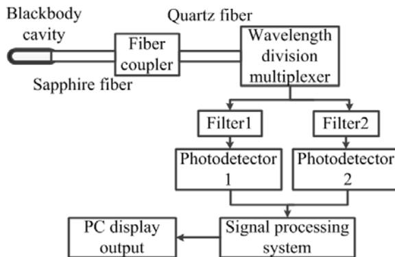
Fig. 4. Colorimetric Measurement System.
