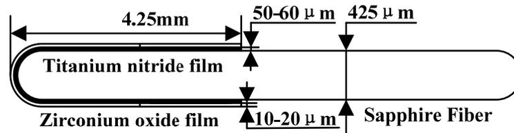
Fig. 2. The Sapphire Fiber Sensor Blackbody Cavity.
