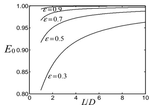
Fig. 3. Optical Fiber Temperature Sensor Cavity Effective Emissivity.
