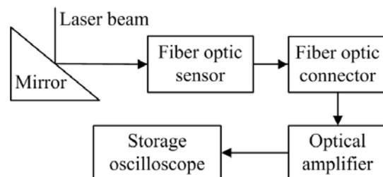
Fig. 6 Dynamic Calibration System.
