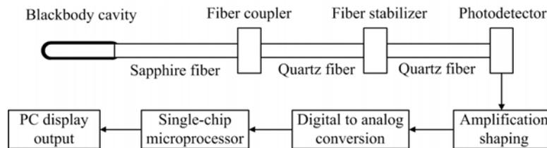
Fig. 1. Sapphire Fiber Sensor Measuring System.
