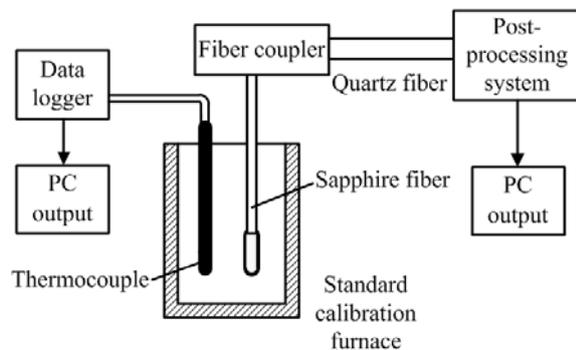
Fig. 5. Static Calibration Device.
