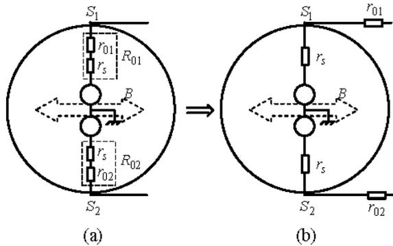
Fig. 3. A model of the electromagnetic flow-meter transducer with electrode fouling. Model (a) can be equivalent to model (b).
