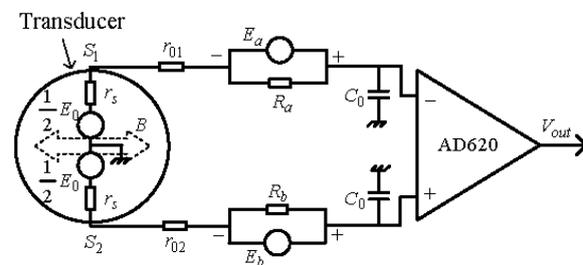
**Fig. 9.** Circuit model of simulation experiment for zero stability.
