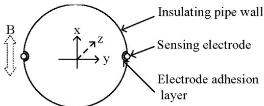
Fig. 1. Numerical Model for the electromagnetic flow-meter with electrode fouling. B denotes the magnetic field.
