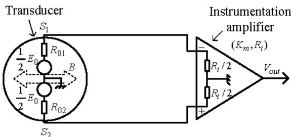
Fig. 4. A model of measurement loop. B denotes the magnetic field.
