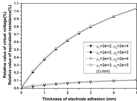
Fig. 2. Virtual voltage (equivalent resistance) between two sensing electrodes versus thickness of electrode adhesion.
