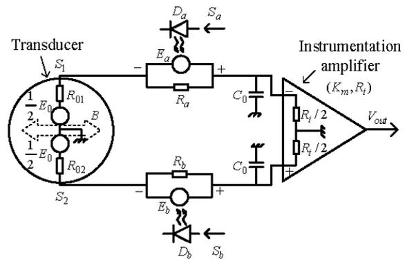
Fig. 5. Principle block diagram of a dual-excited electromagnetic flow-meter based on PV Cell.
