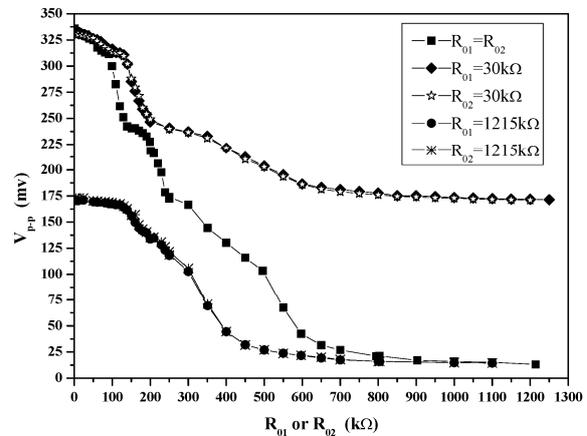
Fig. 8. Variation of  $V_{P-P}$  with  $R_{01}$  and  $R_{02}$  for simulation experiment based on resistors.
