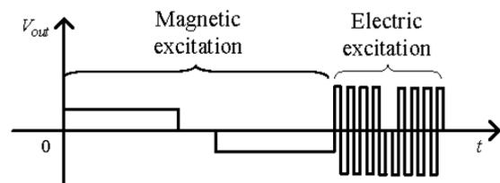
Fig. 6. Illustration of time share of dual excitation in one measuring cycle.  $t$  denotes the time, and  $V_{out}$  denotes the output voltage of the measuring loop.
