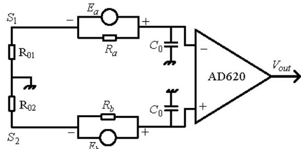
Fig. 7. Circuit model of simulation experiment for electrode adhesion self-diagnosis.
