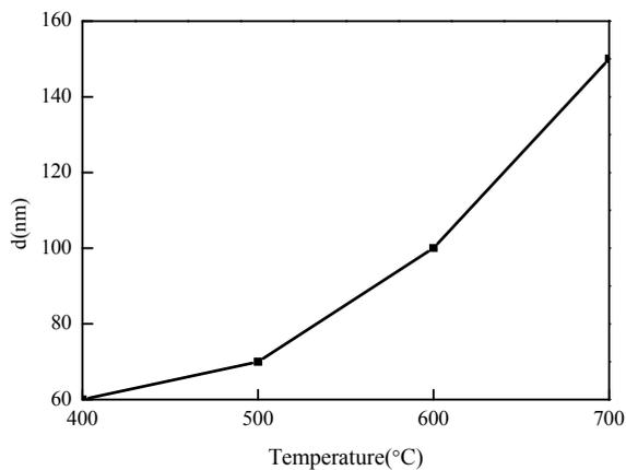
**Fig. 4.** Curve of SnO<sub>2</sub> crystal particle size at different temperatures.
