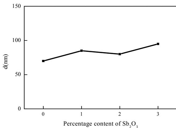
**Fig. 6.** Curve of SnO<sub>2</sub> crystal particle size at different doping Sb<sub>2</sub>O<sub>3</sub>.
