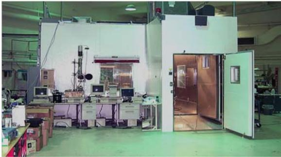
**Fig. 12.** A Photograph of the ECBC Aerosol Sampling Chamber (Aberdeen Proving Ground, MD). Microstructured Arrays Air Filters are placed inside the chamber with three reference filters to determine the particle collection efficiency.
