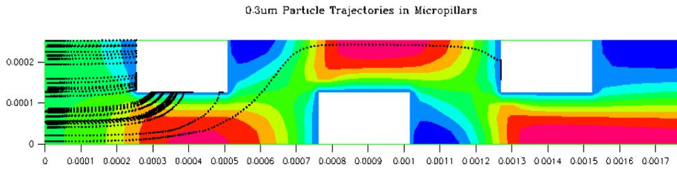
**Fig. 5.** CFD of Impaction of 0.3 Micron Particles on Microstructures with an Electric Field of 1 V/cm. The particle trajectories (black dotted lines) are shown, showing the majority of particles being impacted and captured by the square micropillars (white square impact surfaces).
