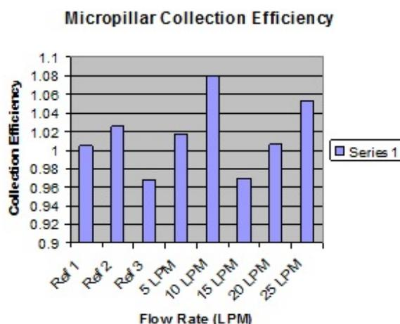
Fig. 15. Coated Micropillar Collection Efficiency Test Results as a Function of Flow Rate.
