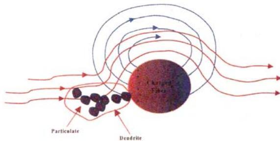
**Fig. 1.** Electrostatic Enhancement of Collection of Particulate with Dendrite Structures on a Single Fiber.
