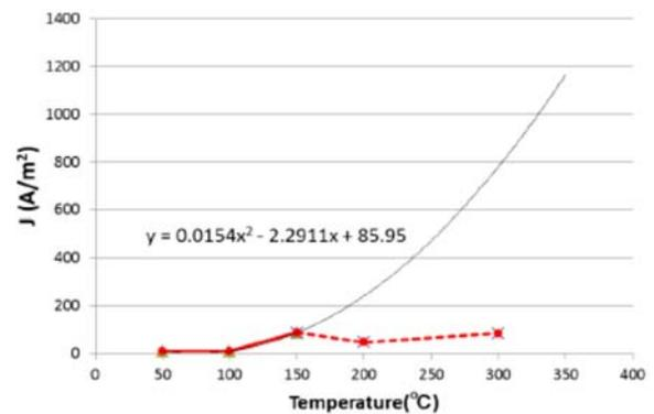
Fig. 7. Modeling of Nano-Boxx Thermionic Emission (dark line) and Experimental Results (Red line).
