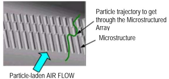
**Fig. 2.** Schematic of Microstructured Array that shows that a tortuous is the only pathway to travel through the Microstructured array filter's impaction surfaces.
