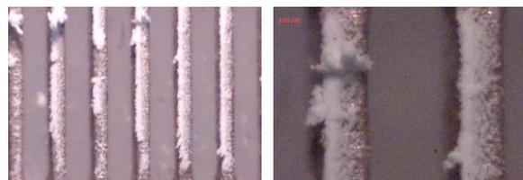
**Fig. 14.** Photographs of micropillars under magnification. Deposited Spheres Creating Dendrites on Micropillars (left). The dendrites on the micropillars shown at different magnification (right).
