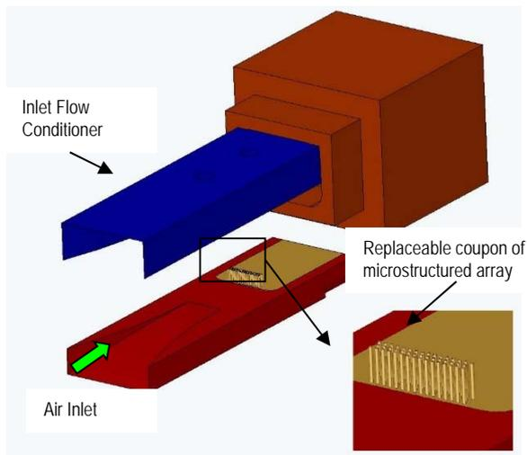
**Fig. 11.** A Micropillar Array Assembly is placed within a larger device to insure good testing procedures.
