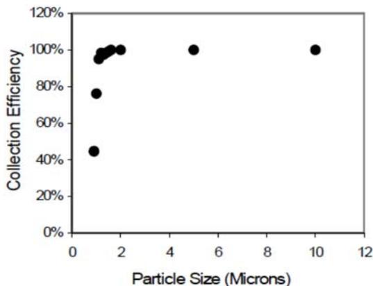
**Fig. 4.** CFD Prediction of Collection Efficiency of Various Particles Sizes without Electric Fields.
