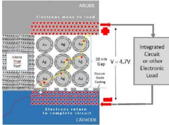
**Fig. 6.** Schematic of Circuit for Thermionic Battery Heat Engine.
