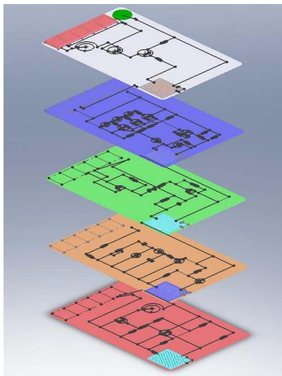
**Fig. 10.** A Schematic of the Compiled Sheet Architecture of the Microstructured Array. Only three layers of microstructured arrays were used for this aerosol collection air testing.
