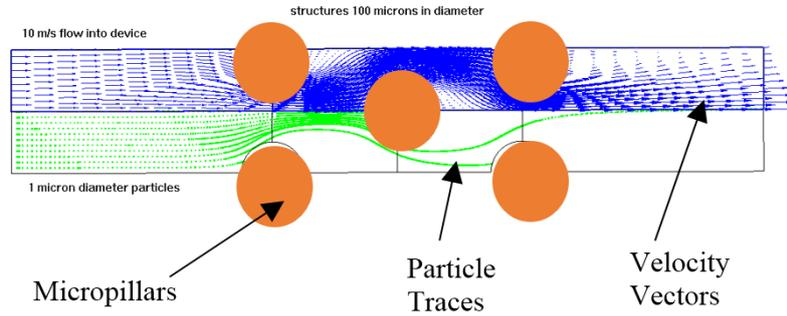
**Fig. 3.** CFD Model of Particle Collection Prediction (as seen from above). Each orange micropillar row is placed to intercept particle traces (green lines) to produce an efficient aerosol collection at a minimum pressure drop (fewer closely-spaced blue lines or velocity traces).
