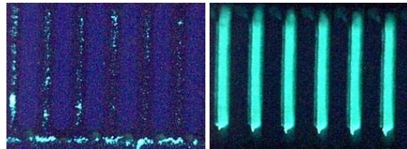
**Fig. 13.** Uncoated (left) and Coated Micropillars (right) with Illuminated Fluorescent Particles.
