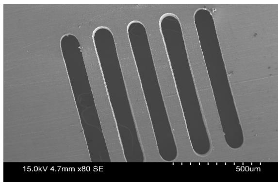
**Fig. 8.** Scanning Electron Micrograph (SEM) of the Microstructured Array Sheet Architecture that Compiles into an Engineering Filter. The 100-micron gaps and micropillars are evident. The next sheet is a spacer with the following sheet similar to above with the micropillars placed such that an unimpeded path through the microstructured array does not exist.
