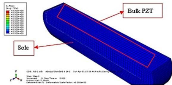
Fig. 4. PZT part and shoe sole part integration for electrical energy harvest.
