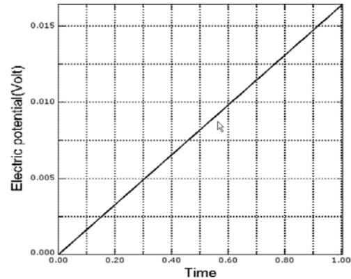
Fig. 6. Rate of change of the electric voltage generated by the PZT.
