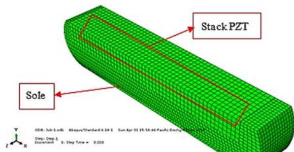
Fig. 5. PZT part optimization for maximum electrical energy harvest.
