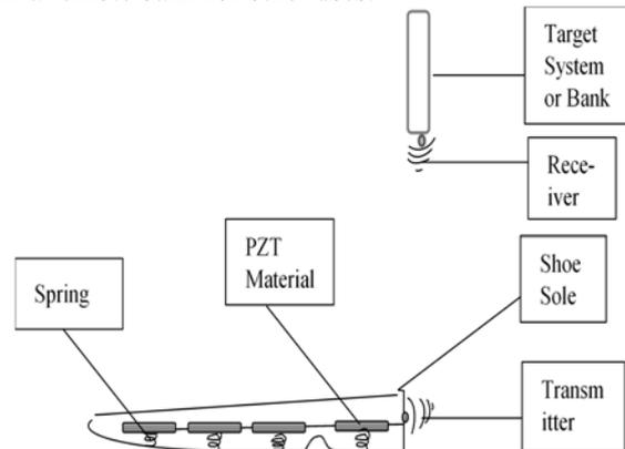
Fig. 1. PZT-integrated shoe sole for electrical energy harvest design concept.
