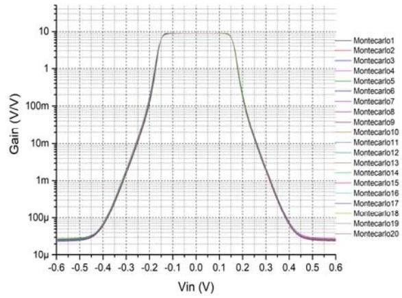
Fig. 8. Monte-Carlo mismatch simulation showing the linearity performance obtained with dynamic base current compensation system.
