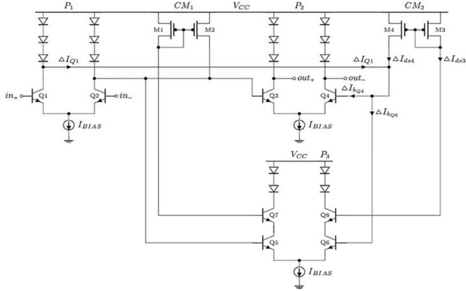
**Fig. 3.** Dynamic base current compensation system for two stages cascaded bipolar amplifier  $P_1$  and  $P_2$ .  $P_3$  operates as a dummy stage used to “monitor” the second stage base current without any degradation of the performances of the second stage itself. Current mirrors ( $CM_1$  and  $CM_2$ ) dynamically replicate 2 times the measured base current.
