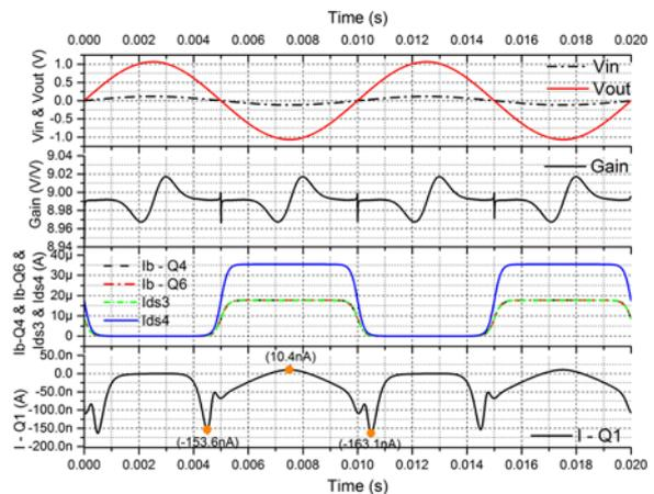
Fig. 7. Dynamic base current compensation performance simulation for 2 cascaded stages of bipolar differential pair with three diodes as loads.
