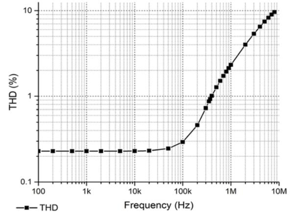
Fig. 6. Pss Simulation – Total Harmonic distortion of dynamic base current compensation system at different frequency.
