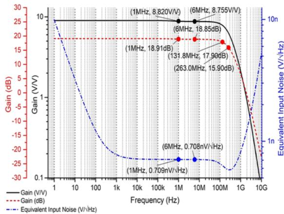
Fig. 4. AC gain and noise simulation for 2 cascaded stages of differential pair with the dynamic base current compensation system.
