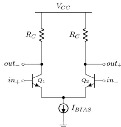
**Fig. 2.** Differential pair with resistive loads.
