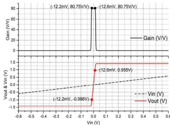
**Fig. 10.** Linearity simulation for 4 cascaded stages of differential pair with dynamic base current compensation system.
