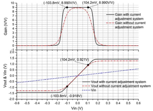
Fig. 5. Simulation – Comparison of linearity performance between 2 cascaded stages of differential pair with and without the dynamic base current compensation system.
