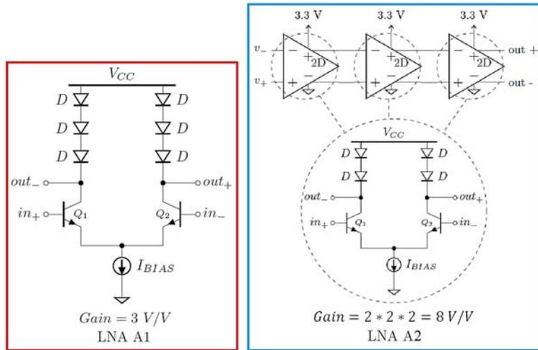
**Fig. 1.** Differential pair with 3 diode<sup>1</sup> loads – LNA  $A_1$  (left); LNA  $A_2$  with 3 differential stages cascaded where each stage with two diodes in series as loads (right).
