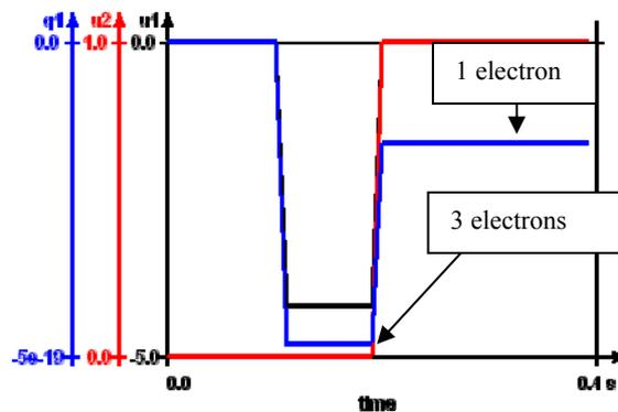
Fig. 6. Storage of one electron in the MTJ/Ring memory.
