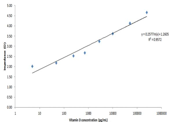
**Fig. 4.** Impedance change according to vitamin D concentration (unit: Ω, concentration: pg/mL).
