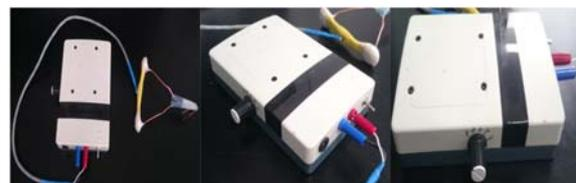
Fig. 3. Vitamin D measurement kit. Vitamin D measurement sensor module applying impedance measurement principle.
