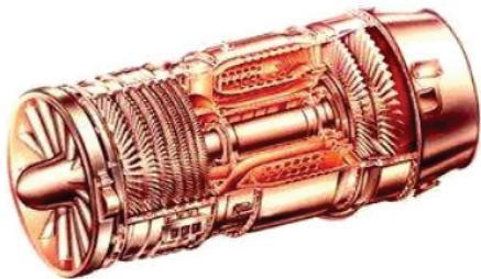
**Fig 7.** J-85 engine cutaway [1].
