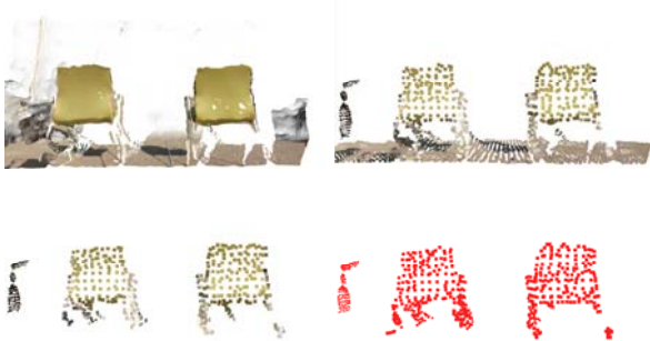
Fig. 2. Results for the four stages of processing. From top-left to bottom-right: original point cloud, down sampled and range limited point cloud, point cloud after ground plane removing and point cloud with detected clusters (two chairs).
