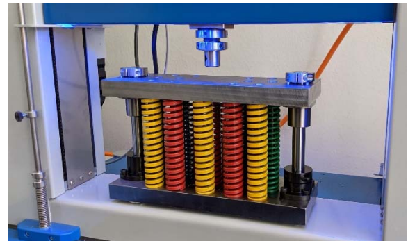
Fig. 1. Modular spring package for investigating changes in stiffness in experiments with force control.
