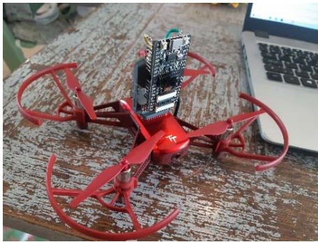
Fig. 3. Our pollination drone carrying the Maix Bit.
