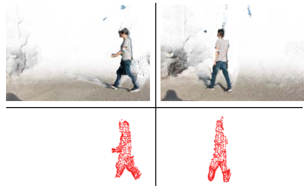
Fig. 3. Moving obstacle detection (wandering pedestrian). In this test, both the person and the AGV are moving. Top: original point clouds; bottom: detected clusters
