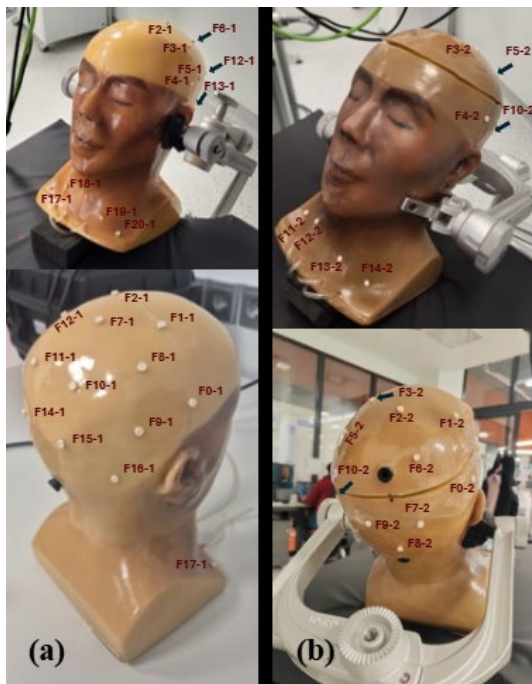
Fig. 2. Head phantoms with circular markers: (a) non-openable phantom with 21 markers and (b) openable phantom with 15 markers. Both are shown in the head holder used for RGB-D imaging.
