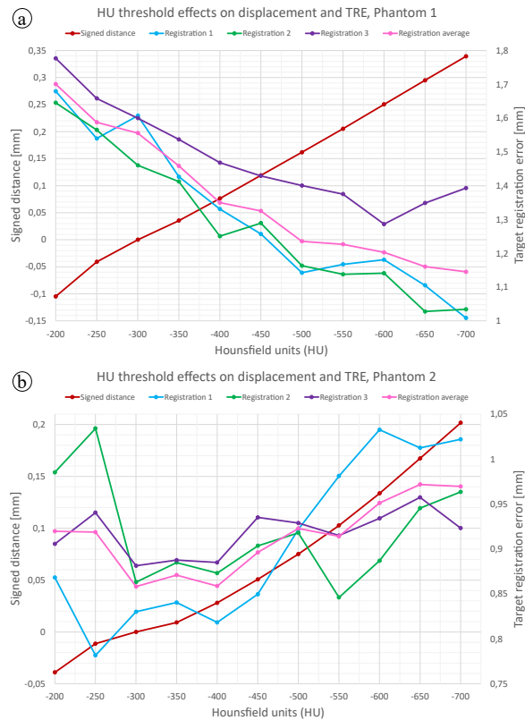
Fig. 3. Mean signed surface displacement (left vertical axis) and target registration error (TRE, right vertical axis) as a function of the HU threshold. (a) Phantom 1: the red curve represents the mean signed surface displacement, where negative values indicate inward surface shrinkage and positive values indicate outward expansion. Lowering the HU threshold value produces a transition from shrinkage to expansion. The blue, green, and purple curves show TRE values obtained from three independent registration sequences (33 registration matrices in total), all exhibiting a decreasing TRE trend with lower HU threshold values. The pink curve represents the mean TRE across all three sequences. (b) Phantom 2: the signed surface displacement follows the same overall trend as in Phantom 1. However, the TRE curves exhibit a less consistent, non-linear behavior across HU thresholds. The averaged TRE curve (pink) indicates a different registration response compared to Phantom 1.
