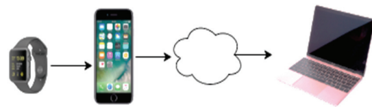
Fig. 1. End-to-end system overview including sensor, mobile phone, internet connection and the server for analysing and login.
