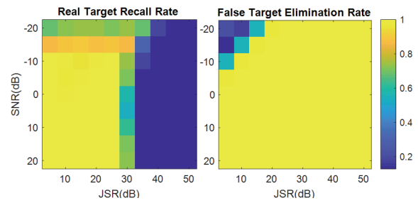
Fig. 2. Visualization of real target recall rate (left) and false target elimination rate (right) of the 4 ISRJ mode under different SNR and JSR conditions.
