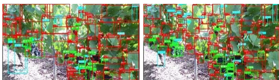
Fig. 4. Example of detection using the combined data fusion and YOLOv5m network trained with RGB images (left) and with RGB-D images (right).
