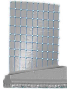
Fig. 7. Arrangement of measurement points on the machined blade.
