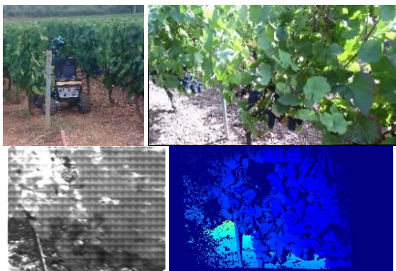
Fig. 1. Top-left: Summit XL mobile robot instrumented with the multi-sensors system; Top-right: RGB image; Bottom left: MS image; Bottom right: Depth image.
