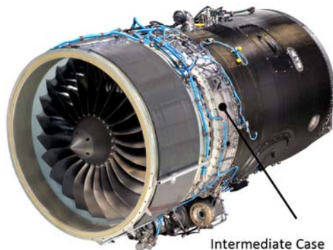
Fig. 1. Pratt & Whitney PW814 aircraft engine, with indication of intermediate case [1].
