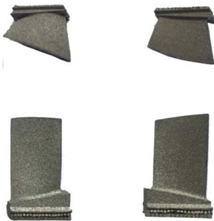
Fig. 1. Blade printed by DMLS method.
