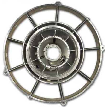
Fig. 2. Intermediate case component of the PW814 engine [1].
