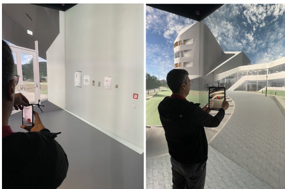
Fig. 3. Experimental setup of user, AR device, tracking targets and CAVE projection of protorealistic 3D models. Left – indoor location using Google ARCore Cloud Anchors API. Right – outdoor location using Google Geospatial Creator.
