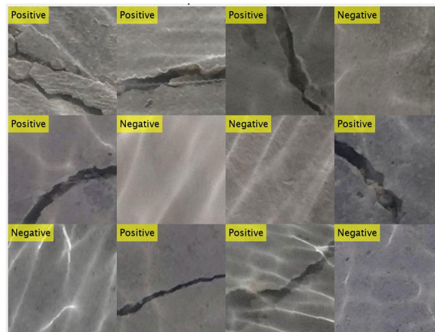
Fig. 1. The Ozgenel's concrete crack dataset augmented by the optical shallow underwater effects.
