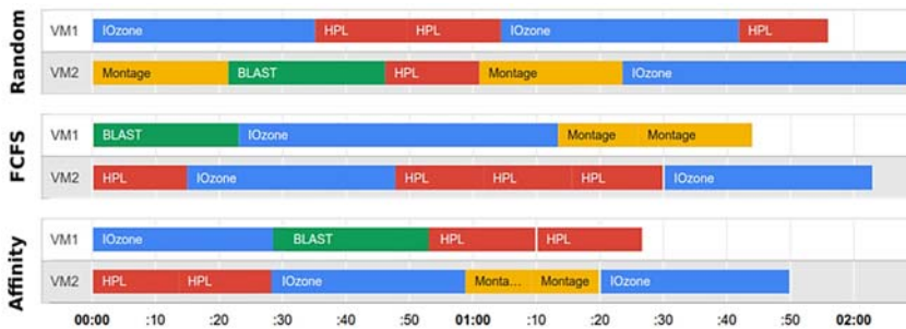
Fig. 5.7. The execution timeline of the queue, in hours, of FCFS, Affinity and Random strategy.
