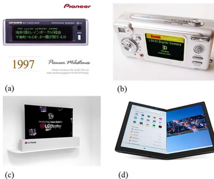
Fig. 1.31. Photographies of selected OLED commercial applications: (a) Car audio system by Pioneer; (b) Kodak digital camera LS633; (c) Rollable 65" OLED TV by LG Electronics, and (d) Lenovo notebook ThinkPad X1 Fold.
