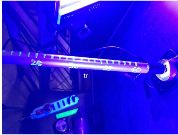
Fig. 5.31. The telescopic rod (tr) is shown, by means of which the distance d between the sensor (se1) of the luxmeter and the PL target can be quickly changed by illuminating the rod with a UV LED lamp.
