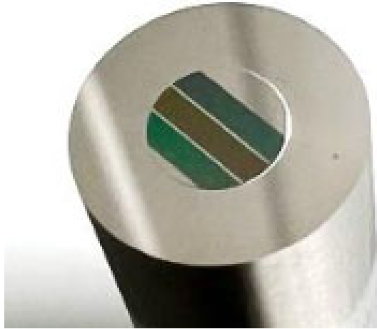
Fig. 3.4. Displays the planar nickel-phosphorus stamp, featuring three distinct grating segments with lattice constants of 1\ \mu\text{m} , 1.5\ \mu\text{m} , and 2\ \mu\text{m} , each with a blazing angle of 60^\circ . These segments were produced using Ultra-Precision Machining (UPM); compare the angle and orientation of the grating grooves with Fig. 3.2.
