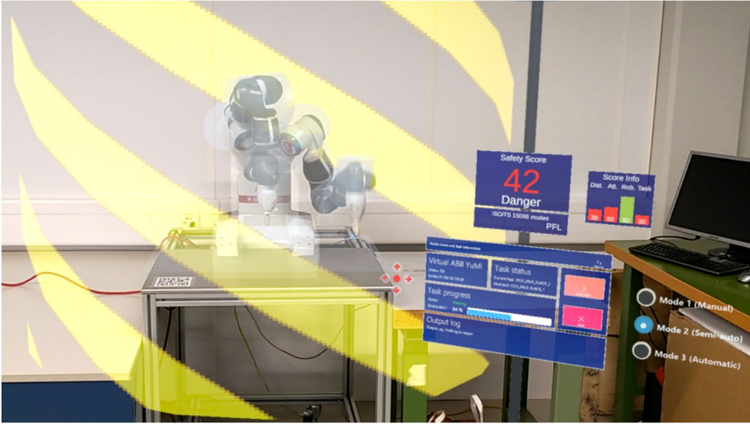
Fig. 2.10. Screen capture of the AR smart glasses during regular human-robot operation. The human operator can visualize in real-time the danger zone, the safety score, and other valuable information.
