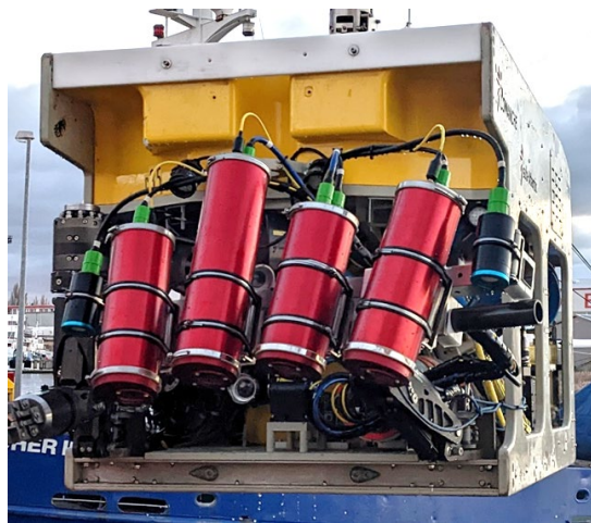
Fig. 1.1. Sensor system mounted on a work-class ROV.
