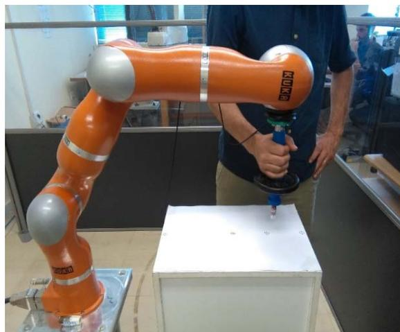
**Fig. 3.** The KUKA LWR robot and the human operator are collaborating to transfer an object (1 kg) [7-8].
