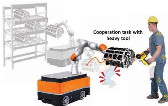
Fig. 4. Example for the repetitive co-manipulation tasks [9].
