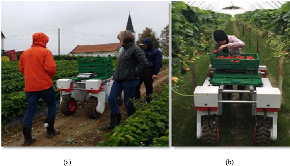
**Fig. 11.** The Thorvald robot in the evaluation environment interacting with the pickers: (a) in the open strawberry fields, (b) in the polytunnel environment [31].
