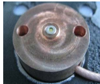
Fig. 7. LD mounted in a copper retainer ring.
