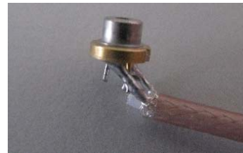
Fig. 6. LD soldered to a formable coax cable.
