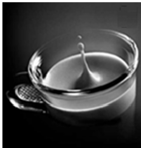
Fig. 7. The formation of a back-moving drop during cumulation (focusing), reflected from the walls of a cylindrical symmetric resonator with a liquid when a drop falls on the liquid surface. It is cos waves, in contrast to sin waves, that accumulate energy, mass and momentum to the center of the hollow acoustic resonator.
