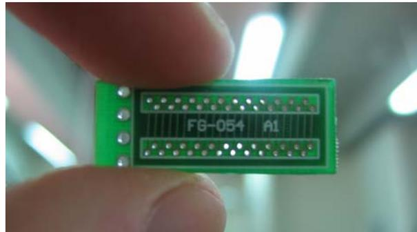
**Fig. 4.** Backlight view of the PCB sensor showing the shape of the embedded Metglas.
