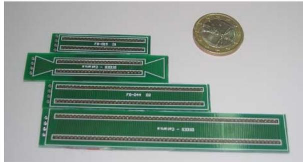
**Fig.3.** Image of a set of PCB integrated Fluxgate sensors.
