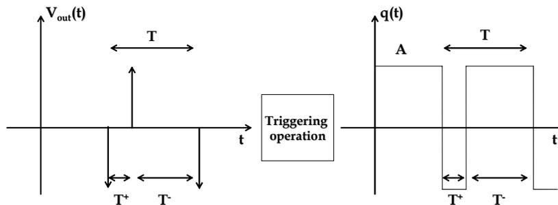
Fig.5. Triggered output waveform retaining the RTD information.
