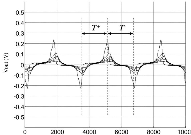
**Fig.2.** Typical pick-up coil output voltage.
