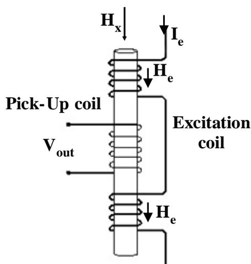
**Fig. 1.** RTD Fluxgate sensor structure.
