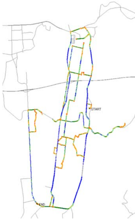
Fig. 1. Target area of about 3 \times 7 km and reference vehicle trajectory. Reference sensor data of total mileage of 31.8 km was acquired.
