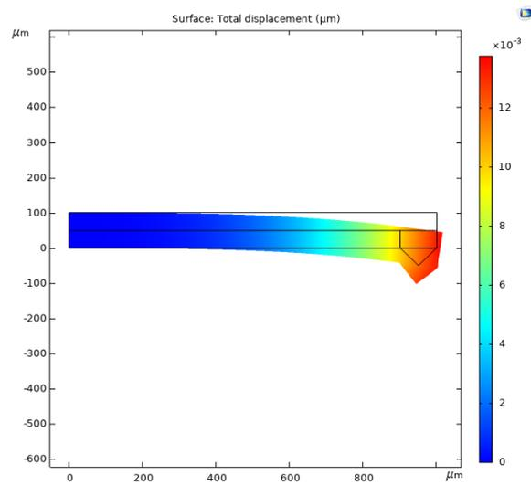
Fig. 9. Displacement of Beam for Nickel as top layer.
