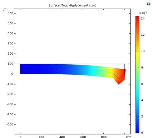
Fig. 7. Total displacement of the Beam for Aluminum as top layer.
