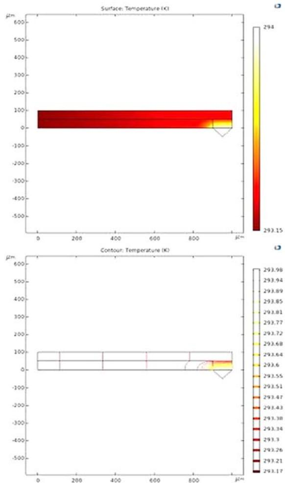
Fig. 6. Temperature gradient across the cantilever beam.
