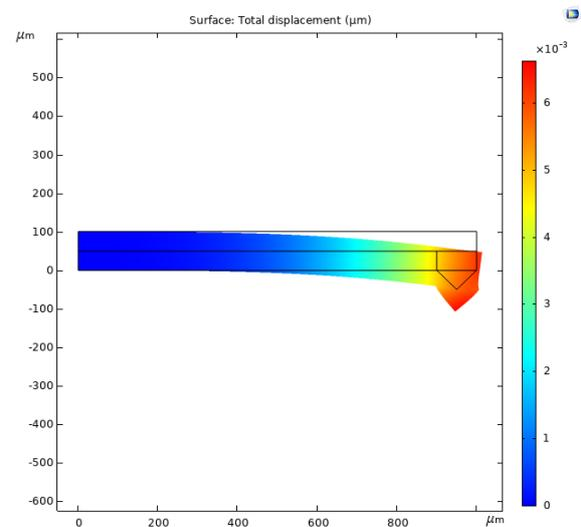
Fig. 10. Displacement of beam for Copper as top layer.
