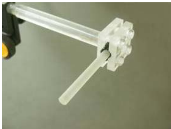
Fig. 16. Magneto-optic element (FR-5) in the holder.
