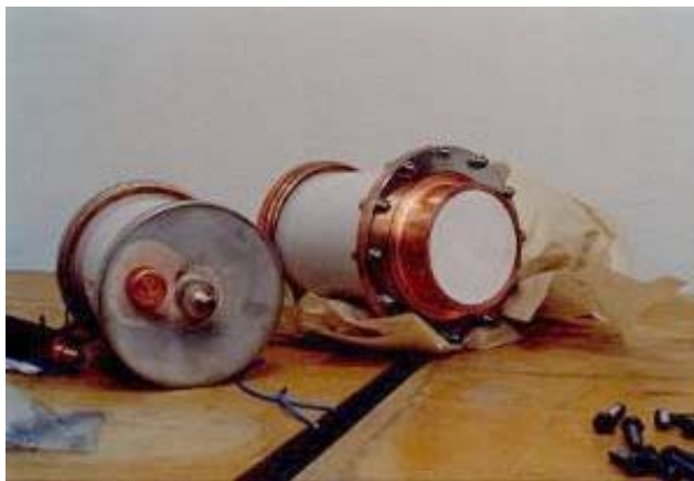
Fig. 6. Experimental construction of vircator, P_{\max} = 250 MW.
