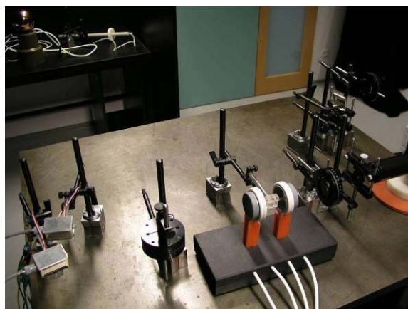
Fig. 17. Experimental setup for high frequency magnetic field measurement.
