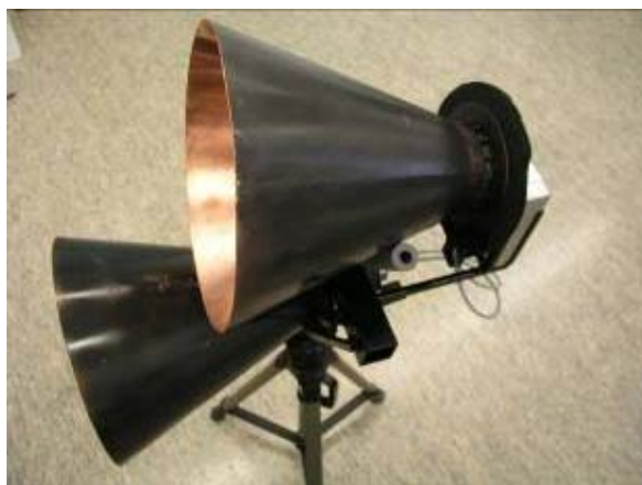
Fig. 12. Realization of optimized combined calorimetric sensor.
