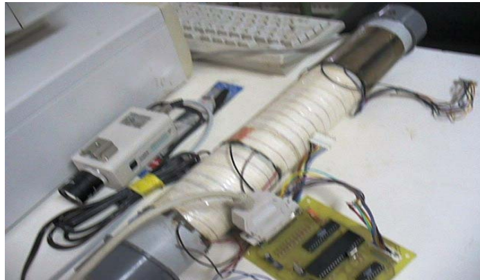
Fig. 2. Electrical Capacitance Tomography sensor.
