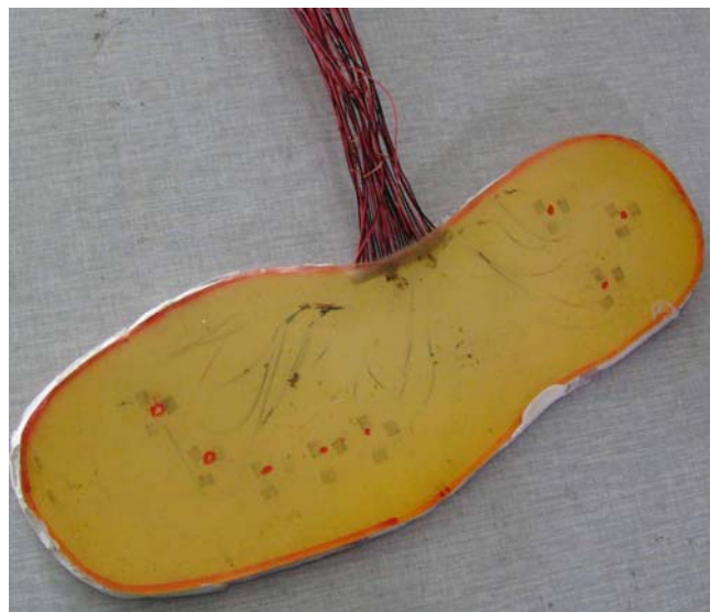
Fig. 3. The picture of actual piezoelectric ceramic sensors distribution inserted into an insole, among them, red points are measurement points and grey points are piezoelectric ceramic sensors distribution place.
