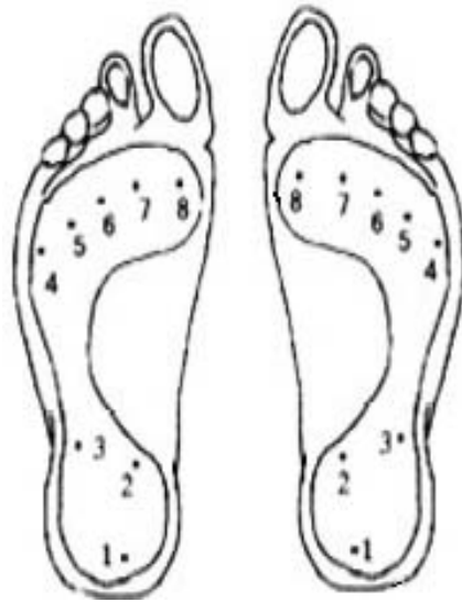
Fig. 1. Measurement points distribution on foot according anatomical structure of foot: HL, heel lateral (1, 3); HM, heel medial (2); M5, metatarsal 5 (4); M4, metatarsal 4 (5); M3, metatarsal 3 (6); M2, metatarsal 2 (7); M1, metatarsal 1 (8).
