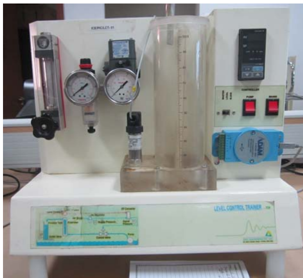
Fig. 3. Level control station.
