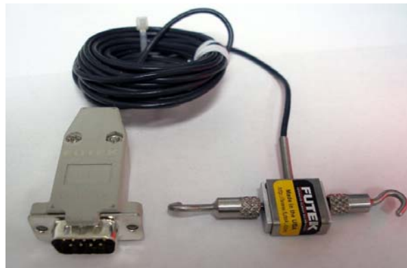
Fig. 2. Futek LSB200- 10 lb S-Beam load sensor interfaced with Dallas 2433 4Kbit chip and male D-sub 9 connector.
