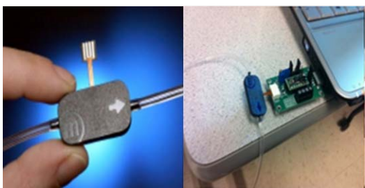
Fig. 8. Disposable microfluidic pump (Bartels Mikrotechnik mp6 Micropump) capable of pumping both air maximum flow: 18 ml/min (300 Hz) and water maximum flow: 7 ml/min (100 Hz).
