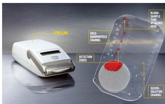
Fig. 2. Lab-on-a-chip with external automation [115].
