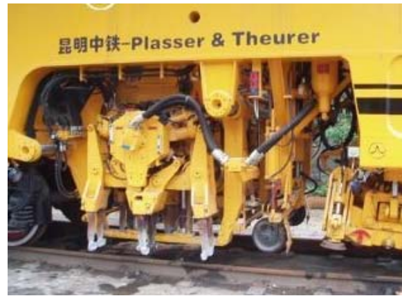
Fig. 5. The tamping unit of the ballast temper.
