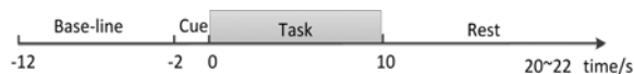
Fig. 1. The event procedure during a trial. In our experiment, the time duration of a trial is much longer than other EEG based experiments. The reason for this is that we acquire functional near-infrared spectroscopy (fNIRS) signals simultaneously with EEG signals. Due to the nature of hemodynamic responses, fNIRS signals take much longer time to return to the base line than EEG signals.
