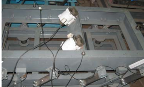
Fig. 2. Harmonic vibration synchronously test bench that driven by two exciting motors.
