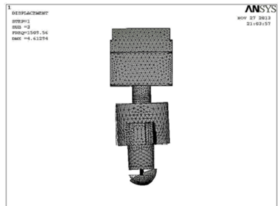
Fig. 5 (c). The third order vibration and deformation
