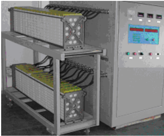
Fig. 8. The test platform of lead-acid batteries intelligent management system.
