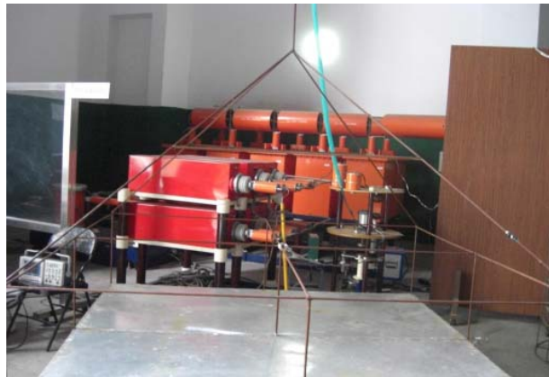
Fig. 7. The sketch map (left) and photo (right) of the complicated steel frame used for test and verify the accuracy of the magnetic steel rods method.
