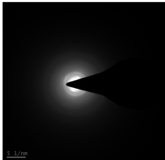
Fig. 3. SAED patterns of prepared ZnO nanopowder.
