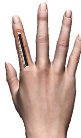
Fig. 2. An RFS can measure the flexion/extension of the joint when lied down on-top of the joint itself. In this picture a FP RFS on-top of the proximal-interphalangeal joint of the index finger.
