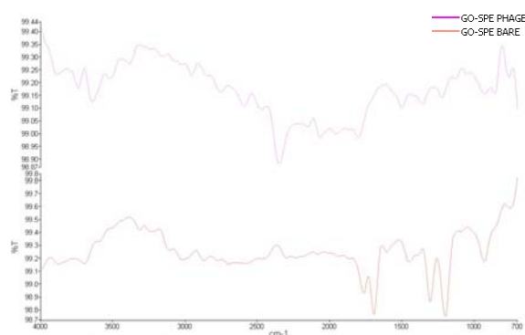
Fig. 2. FTIR spectra of bare GO-SPE and GO-SPE/Phage.
