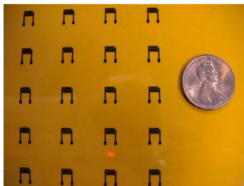
Fig. 5. Fabricated humidity sensor on flexible polyimide substrate.
