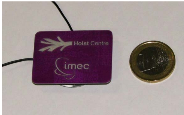
Fig. 1. Thermoelectric module having a thickness of three Euro coins for integration in a piece of clothing.
