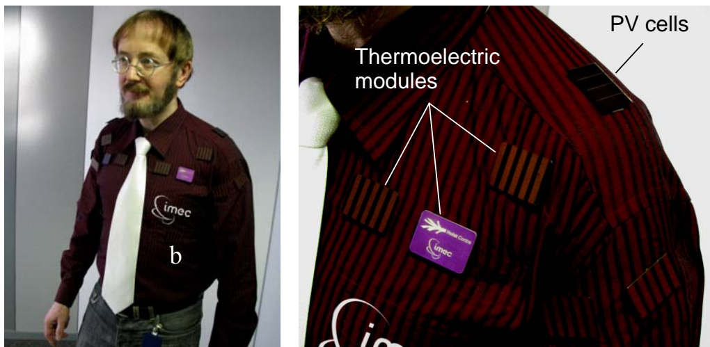
Fig. 2. Electrocardiography shirt and some of its modules. The TEG modules are chameleon-like painted for invisibility. The only one of modules has a different color to give an idea about its size.
