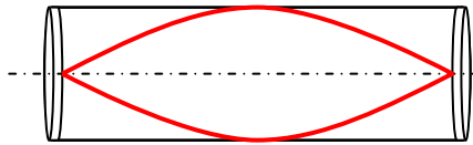
Fig. 1. 1 st harmonic for a closed-end air column.
