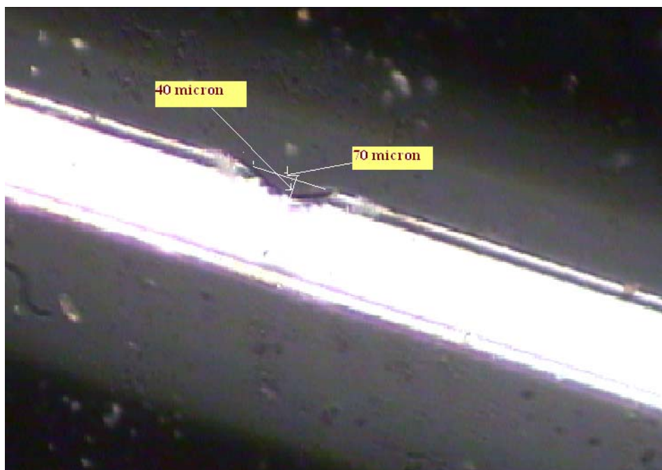
Fig. 2. V-Groove fabricated in LMA-PCF.
