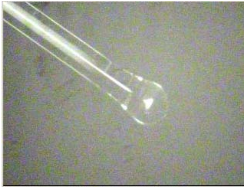
Fig. 8. Ball lens fabricated on tip of PCF.
